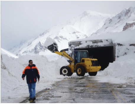
Even in avalanche areas snow has been easily removed due to anti-icing.
