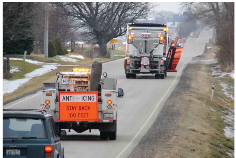
Anti-icing roadways prior to an event in McHenry County, Illinois. (Photo courtesy of Mark DeVries)
